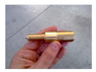
3 The nozzle can be further disassembled from the assembly by means of a no. 2 Allen wrench.
